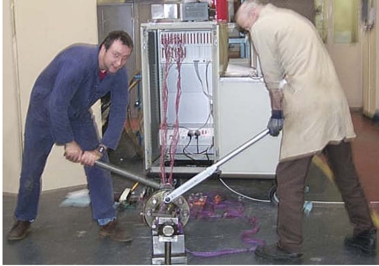
Fig. 4. Arrangement for gasketed flange joint assembly.
